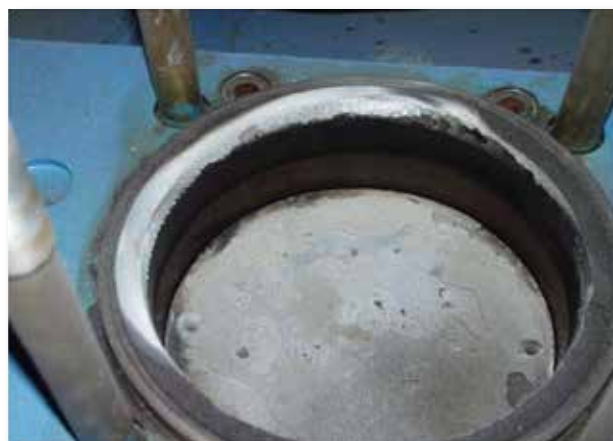
Silica deposits at a cylinder and valve of a thermal power station run with biogas
